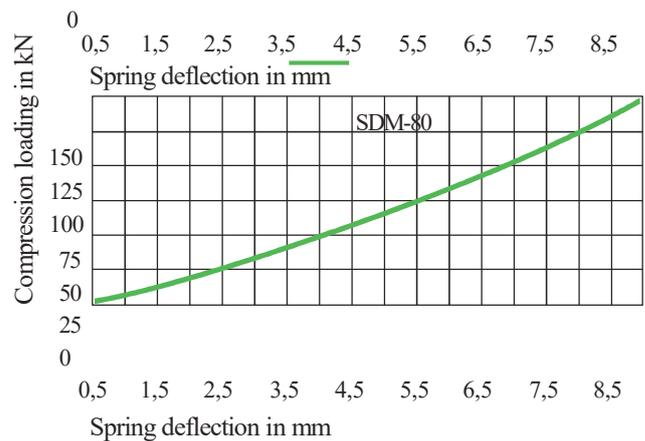
In the case of the Silent Delta SDM-P double element, the spring deflection is doubled for the same loading.
