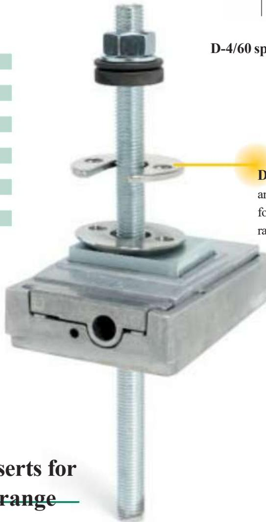
D-4/60 spacing washers are practical assembly aids for extending the adjusting range. They can be easily inserted later on and provide a secure position thanks to push-in cams.
