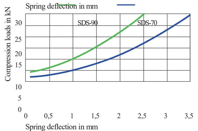
In the case of the Silent Delta SDS-P double element, the spring deflection is doubled for the same loading.
