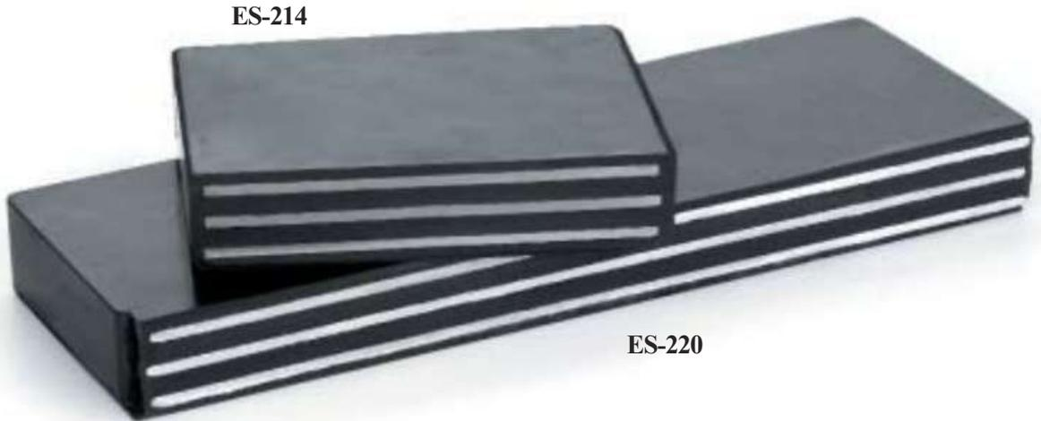
The layering of sound non-absorbent (e.g. metal) and sound absorbent (e.g. rubber) materials results in additional reflection damping (see page 31). With a low degree of deflection, the layer achieves the best possible degree of damping for the smallest possible compliance. Layers are suitable for loads of 300 to 800 N/cm<sup>2</sup>.
